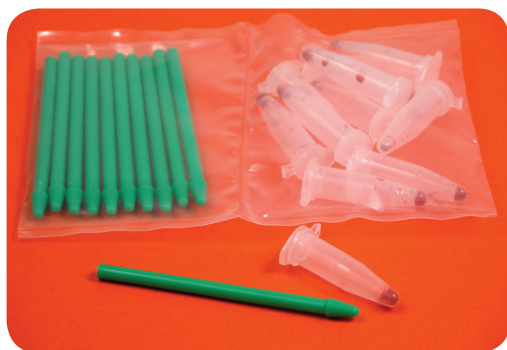
Figure 26: EZ-Grind™ showing pestles and prepacked grinding resin.
