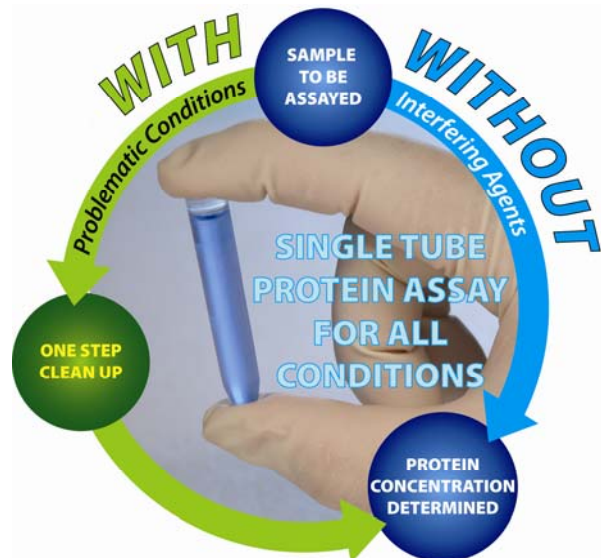
Figure 1: CB-X™ Protein Assay Scheme. Protein samples are rapidly assayed with a single reagent with in five minutes. In most cases the assay will generate accurate results, however if interfering agents are present artifactual results may occur. In this situation the samples are cleaned with a one-step procedure in a single tube. This generates accurate protein estimations.
