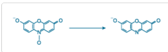
Conversion of alamarBlue dye from oxidized to reduced form
